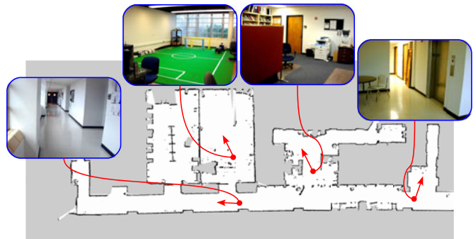
Fig. 6. Occupancy-grid map of the third floor of the CS department with 13 faculty offices, three research labs, a conference room, and a common area with a kitchen.
